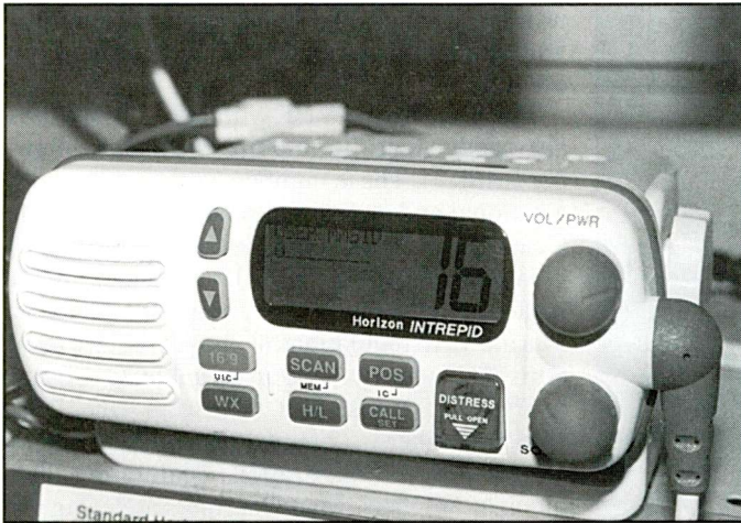
An inexpensive DSC marine radio with the big red distress button cover located on the bottom.
