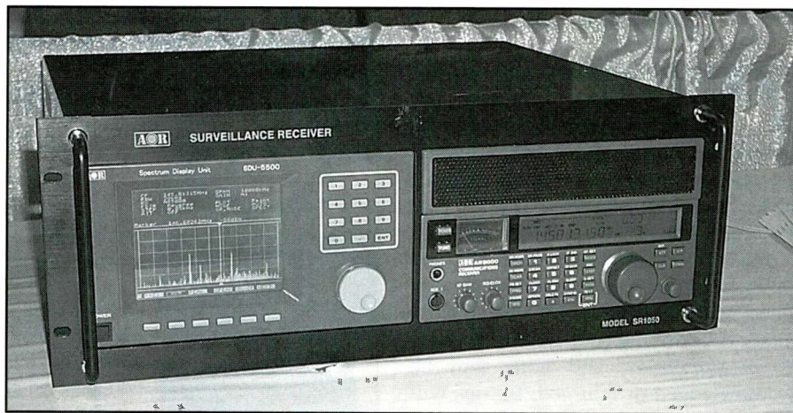
While not new, this was the first time I had seen one of these up close. It's a cabinet that houses the AR-5000 +3 receiver alongside an SDU-5500 spectrum display unit. It's a completely functional and extremely fun to play with package!
