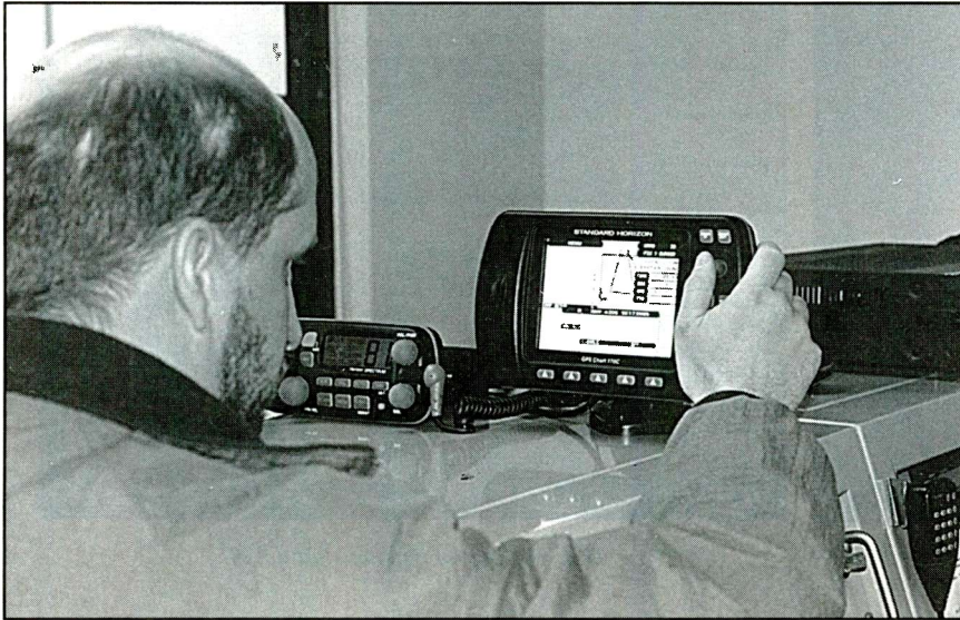
The Coast Guard Auxiliary tests DSC and position polling with 100 percent success.
