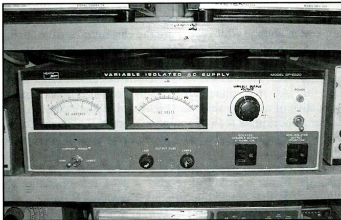
Heath's SP-5220 variable AC supply is the answer to workbench clutter! AC voltage and current metering, overload protection, isolation transformer, and a variable autotransformer are housed in a single compact enclosure. The meter scales on this Heath are large and easy to read.
