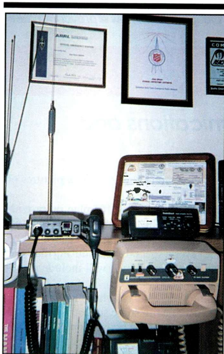
Here is the RadioShack TRC-511 in use in the shack, left center. We told you it's small! Notice the vintage Johnson Messenger 130A, still in active service, lower right. (Photo by N3HOE)
