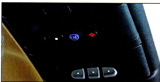
Close-up of the OnStar control head mounted in a ceiling console. (Photo courtesy of OnStar)
